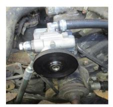
Start the engine, keep the fluid level topped up to the max level, check for any leaks, tighten connections if necessary.
